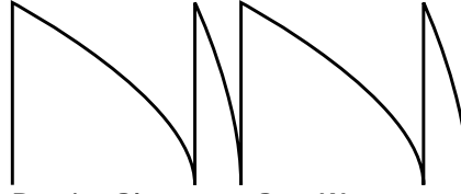
Positive Skew on a Saw Wave
